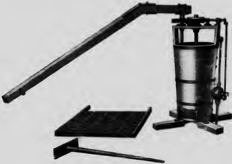
Egeberg peat pulping machine operated by horse-power.
